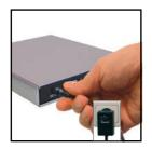
2. Connect the cable of the power supply to the Freecom Mobile DVD RW Recorder and the power supply itself to the socket.
